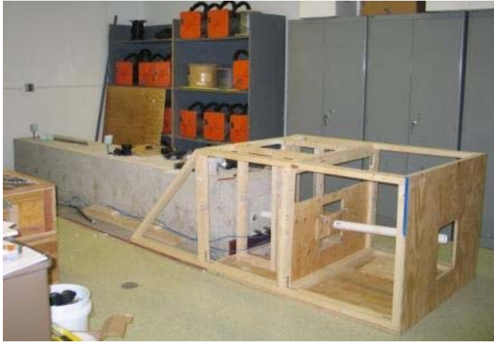
a. 2 ft x 2 ft x 12 ft concrete block and attached testing frame.
