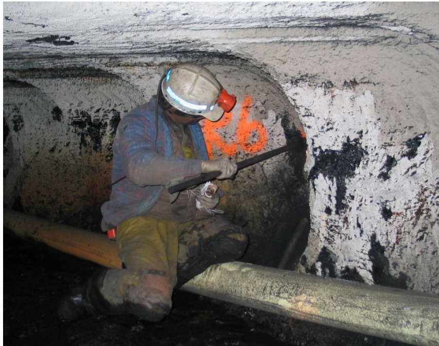
Figure 9.10 Clean blasting hole R6 for reflection test.
