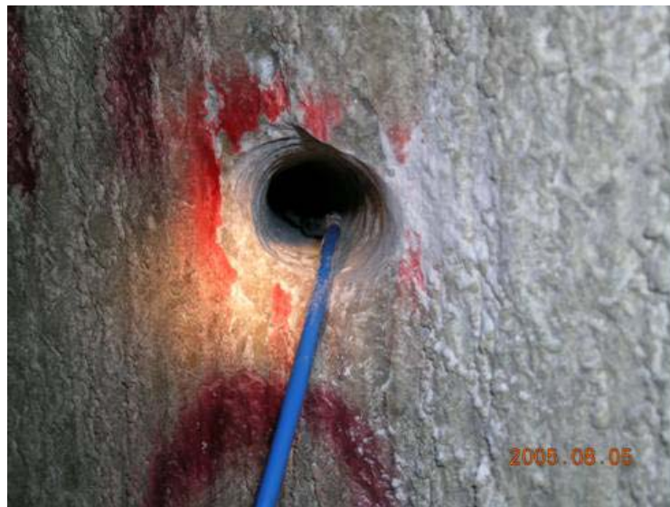
Figure 8.4 Retrievable sensor was installed in the sensor hole used five months earlier.
