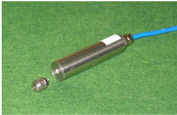
Figure 2.1 A retrievable uniaxial sensor consists of a sensor body and a sensor anchor made of a screw assembly.
