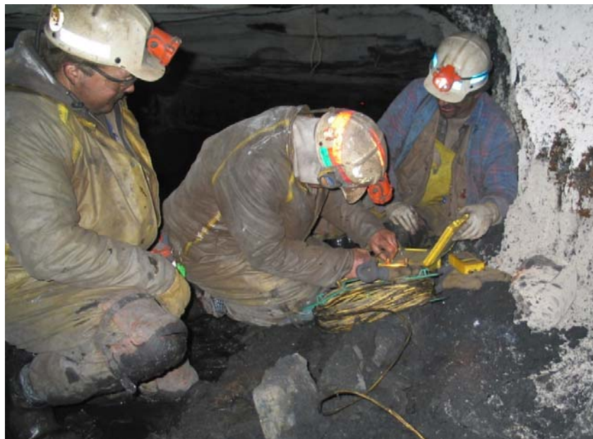
Figure 9.12 Preparing the detonation.
