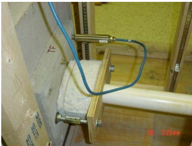
c. Sensor and testing panel installed at the front of the concrete block.
