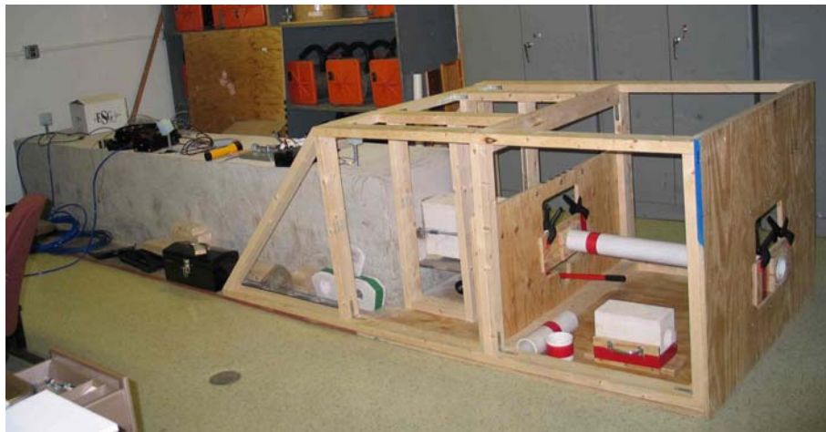
Figure 2.28 Concrete block and borehole support frame for 3D sensor testing.
