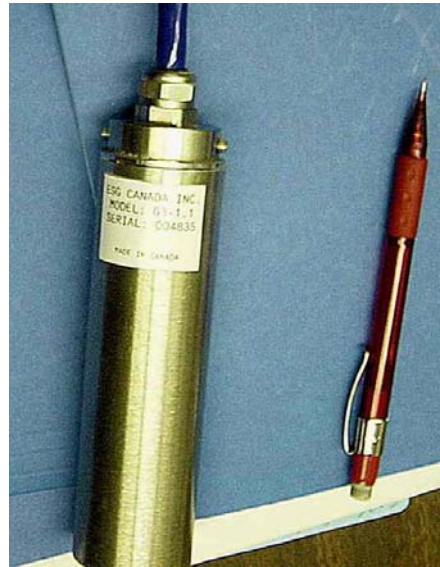
Figure 2.26 A three-dimensional accelerometer.
