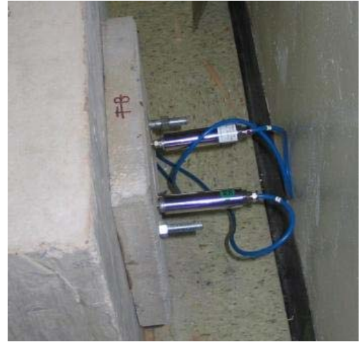
b. Sensors and sensor panel attached at the rear end of the block.
