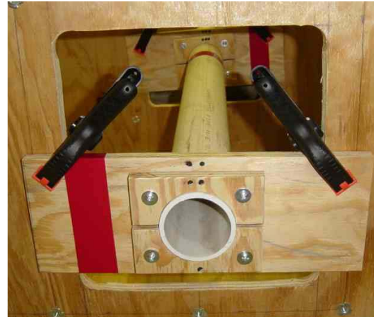
b. Specially designed borehole system.
