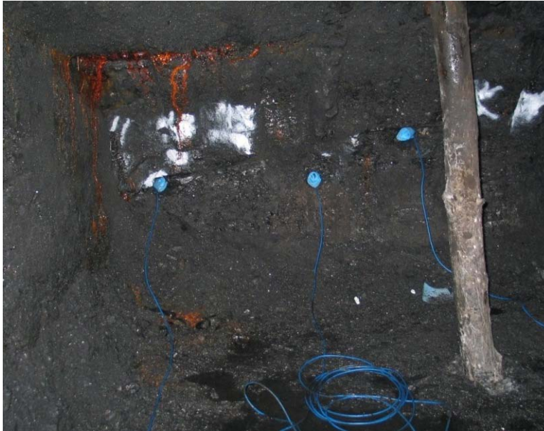
Figure 9.17 Sensor holes were sealed with the blue foam to prevent the interference by shock waves (picture was take at testing site II, Harmony Mine).
